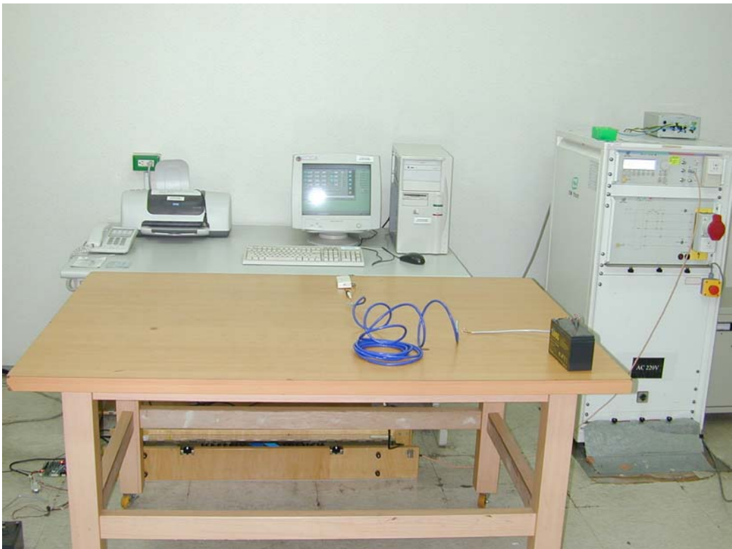
EFT/B Test Setup – Clamp (Signal Cable)
